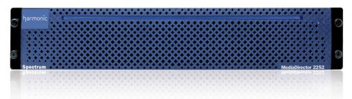
MediaDirector™ 2252 system controllers are the core of the Spectrum™ media server system, actively managing the flow of data to and from other Spectrum components, such as MediaStore™ 5000 storage arrays and MediaPort™ 7000 media I/O modules. MediaDirector 2252 provides 16 high-speed media I/O ports and the necessary processing power to support a wide range of configurations and workflows. Its SAS interface provides redundant data paths between the MediaDirector and MediaStores.
